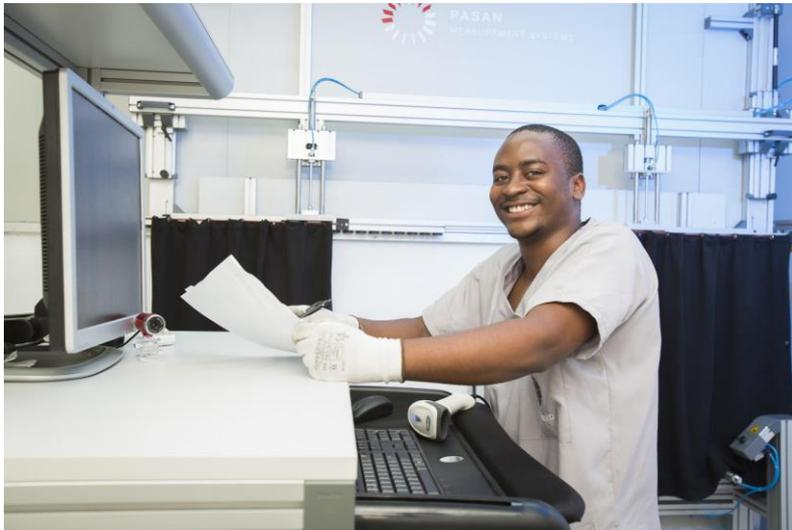
The sun-simulation test (left) confirms the power of a module under accurately controlled IEC defined temperature and illumination conditions. ARTsolar uses the industry leading Pasan testing machine which has been proven to provide more accurate power of the module. For the customer's benefit, ARTsolar then rounds the power down the the nearest 5W. So a 319Wp module will be labelled as 315Wp.
